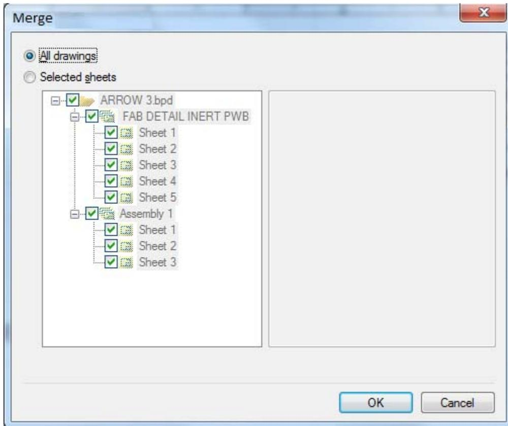
The user is warned if the CAD data source is not identical (file name and date) for both BPD files. The drawing sheets that are appended to the currently open BPD file will be refreshed with the CAD data from the current BPD file.
